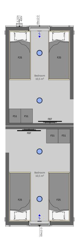
EV32 is a functional EVAC module with two bedroom. Can be connected to other our EVAC and site hut modules, especially with the modules EV31HCR and EV31HCL
