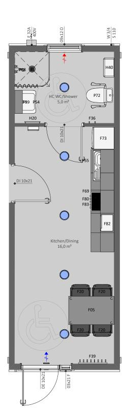
**EV31HCL** is a functional EVAC module with kitchen/dining room and handicap WC with a shower. Can be connected to other our EVAC and site hut modules, especially with the module EV32
