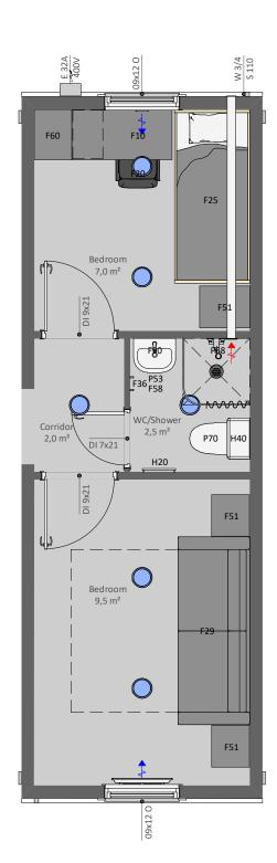
**EV23R** is a functional EVAC module with two bedrooms, corridor and WC with a shower. Can be connected to other our EVAC and site hut modules, especially with the module EV21RE
