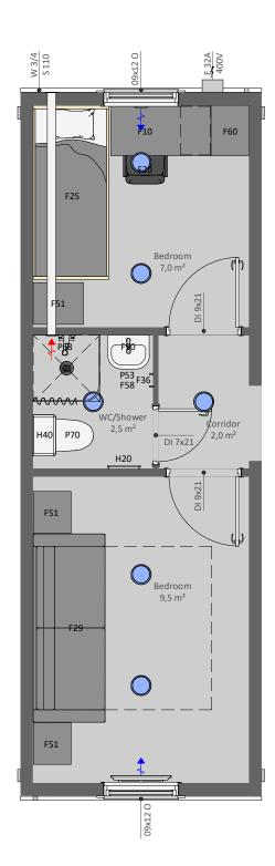
**EV23L** is a functional EVAC module with two bedrooms, corridor and WC with a shower. Can be connected to other our EVAC and site hut modules, especially with the module EV23LE
