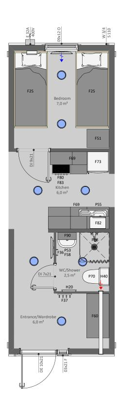
**EV21RE** is a functional EVAC module with one living/bedroom, kitchen with dining area, WC with a shower and an entrance/wardrobe room. Can be connected to other our EVAC and site hut modules, especially with the module EV22R and EV23R
