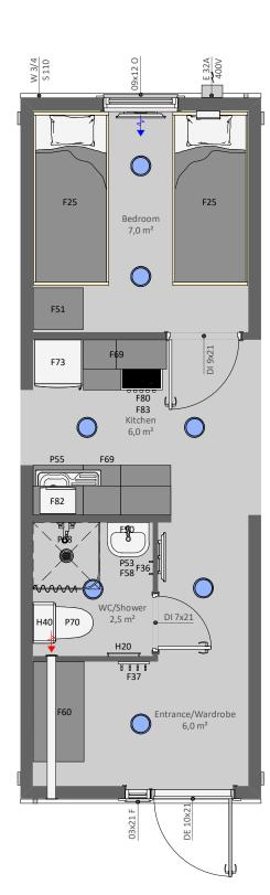
**EV21LE** is a functional EVAC module with one living/bedroom, kitchen with dining area, WC with a shower and an entrance/wardrobe room. Can be connected to other our EVAC and site hut modules, especially with the module EV22L and EV23L
