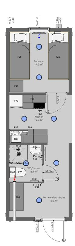
**EV21L** is a functional EVAC module with one living/bedroom, kitchen with dining area, WC with a shower and an entrance/wardrobe room. Can be connected to other our EVAC and site hut modules, especially with the module EV22L
