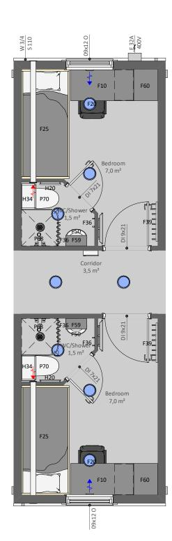
**EV01L** is a functional EVAC module with two bedrooms, two WC with a shower and a corridor in the middle of the module. Can be connected to other our site hut modules
