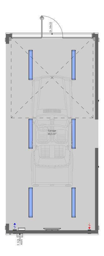
GA10WR is a single open space wide garage module without a wall on one long side, can be connected to other our site hut and garage modules
