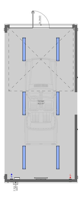
GA10WHR is a single open space wide and high garage module without a wall on one long side, can be connected to other our site hut and garage modules
