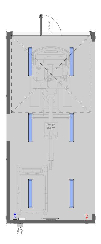
GA10WHL is a single open space wide and high garage module without a wall on one long side, can be connected to other our site hut and garage modules
