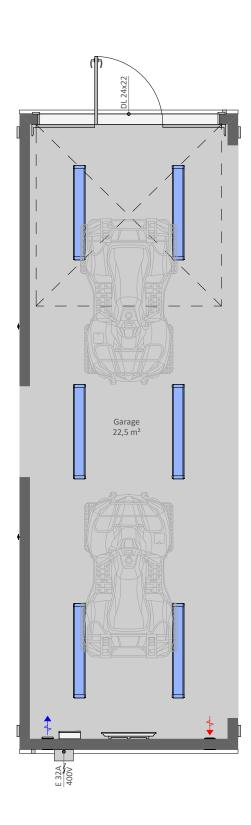
GA10L is a single open space garage module without a wall on one long side, can be connected to other our site hut and garage modules
