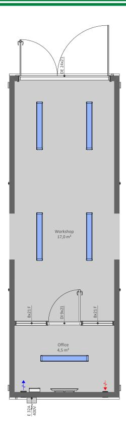
WS21G is an open space workshop module with one office room, can be connected to other our site hut modules
