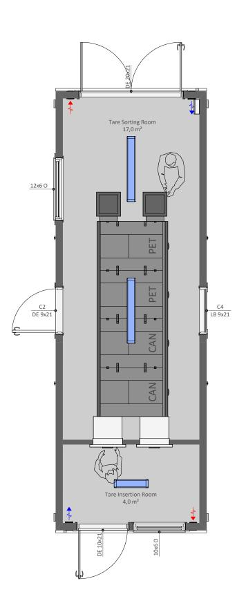
TARE2 is a stand alone tare collection and sorting module with tare insertion room, can be connected to other our site hut modules
