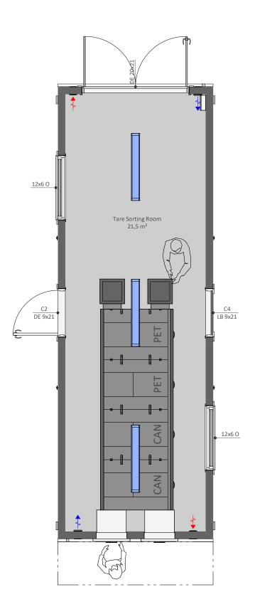
TARE1 is an open space stand alone tare collection and sorting module, can be connected to other our site hut modules
