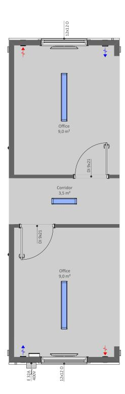
K12VD2 is a open space office module with two office rooms and corridor, without a wall on one long side
