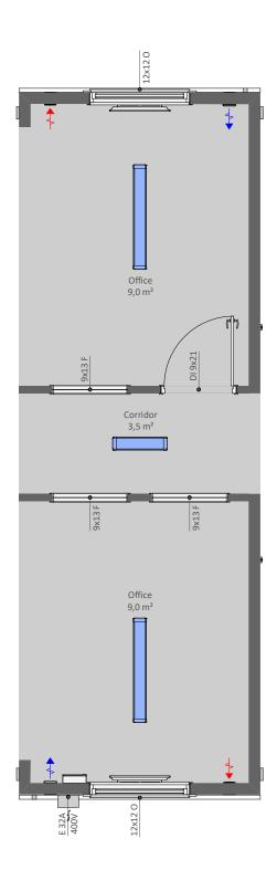
K12HG3D1 is a open space office module with two office rooms and corridor, without a wall on one long side
