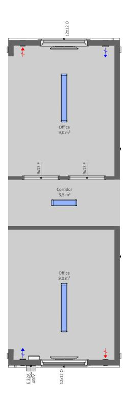
K12HG2 is a open space office module with two office rooms and corridor, without a wall on one long side
