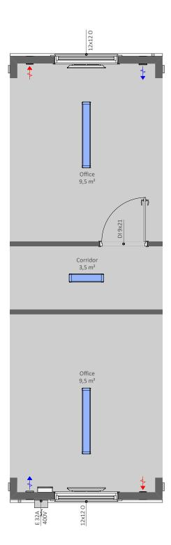
K02D1 is a open space office module with two office rooms and corridor, without walls on the long sides
